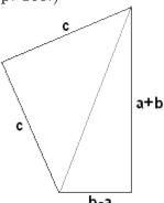
This one comes courtesy of Douglas Rogers from his extensive collection. As in Proof #1, the triangle is rotated 90 degrees around one of its corners, such that the angle between the hypotenuses in two positions is right. The resulting shape of area  $b^2$  is then dissected into two right triangles with side lengths (c, c) and (b - a, a + b) and areas  $c^2/2$  and  $(b - a)(a + b)/2 = (b^2 - a^2)/2$ :
