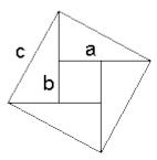
The square has a square hole with the side (a - b). Summing up its area  $(a - b)^2$  and 2ab, the area of the four triangles  $(4 \cdot ab/2)$ , we get
